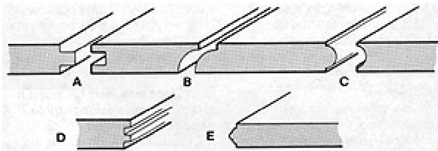
**Figure 5-8.** Molder knives that produce these joints are purchased in sets: (A) tongue-and-groove; (B) drop leaf table; (C) flute and nosing. Examples of full profile cuts: (D) glue joint and (E) cloverleaf.
