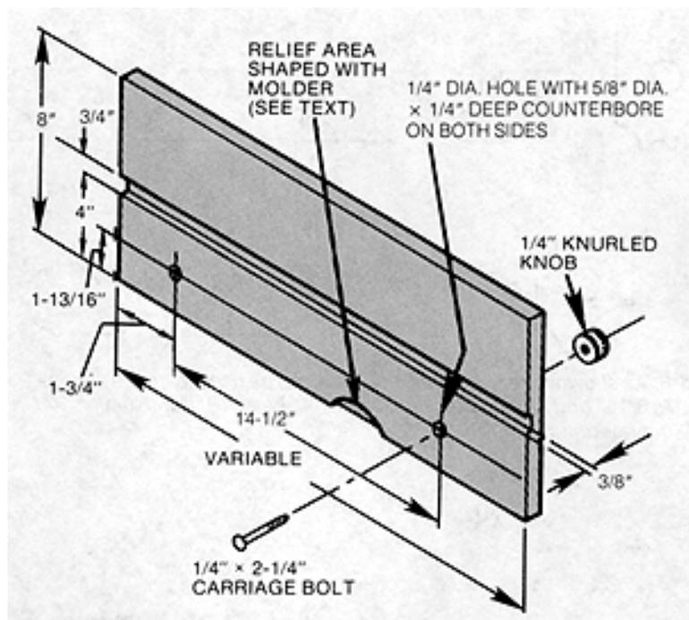
**Figure 5-10.** Construction details of the rip fence extension. If you counterbore for the bolt heads on both sides of the fence, you'll be able to attach it on either side of the rip fence for use on the left or right side of the table.
