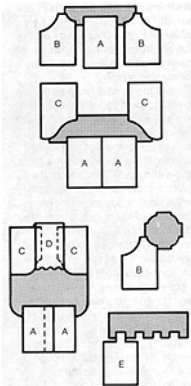
**Figure 5-9.** These shapes are typical of advanced work you can do with the molder head accessory. The shapes of different knives combine to produce the final form. Work like this should be planned in advance, on paper, using the knives as templates: (A) 1" jointer; (B) combination 1/2" and 1/4" quarter-round; (C) ogee; (D) three-bead; (E) groove (part of the tongue-and-groove set).
